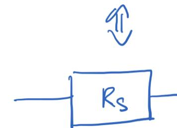
$$R_S = R_1 + R_2 + \dots + R_N$$
